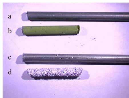
Figure 1. a. Fe rod; b. Fe in PBS for 1-week at 37 °C; c. Mg alloy rod; d. Mg alloy in PBS for 1-week at 37 °C.
