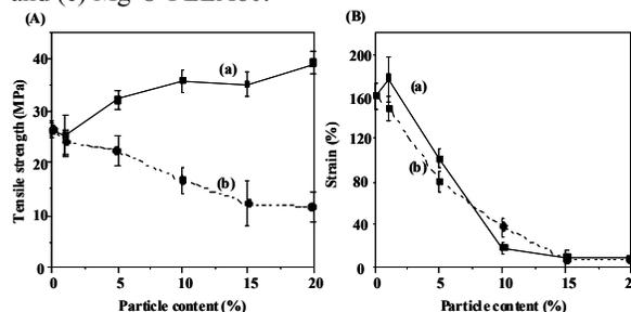
Fig. 2. Dependence of (A) tensile strength and (B) strain on nanoparticles contents within PLLA matrix: (a) Mg-O-PLLA80 and (b)  $Mg(OH)_2$  particle.
