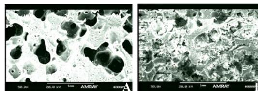
Figure 1. SEM micrograph of uncoated scaffold (A) and calcium coated scaffold (B) (scale bar = 1 mm).
