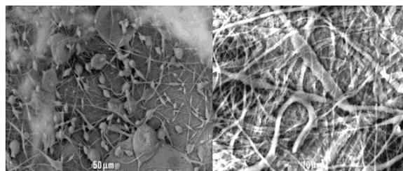
Figure 2. Scanning Electron Microscopy (SEM) of PLA-Silver fibers.
