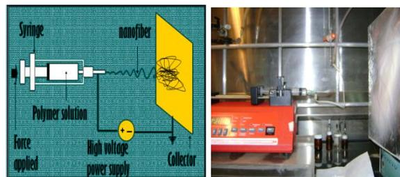
Figure 1. Polymer fibers electrospinning
