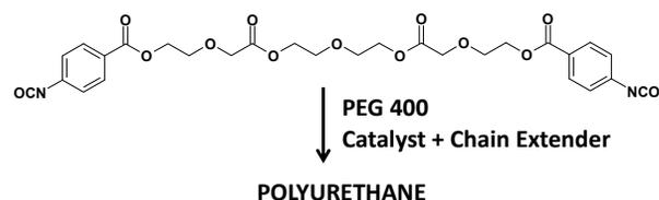
**Figure 3** Absorbable polyurethane polymers for lyophilized foams for wound healing
