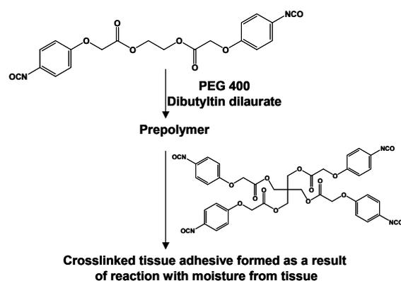
**Figure 2** Absorbable crosslinked polyurethane based tissue adhesive
