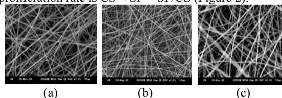
Fig. 1. SEM micrographs of (a) CS, (b) SF, and (c) CS/SF nanofibers.
