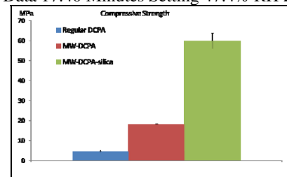
Figure 3. Compressive Strength of Regular DCPA, MW-DCPA and MW-DCPA-Silica
