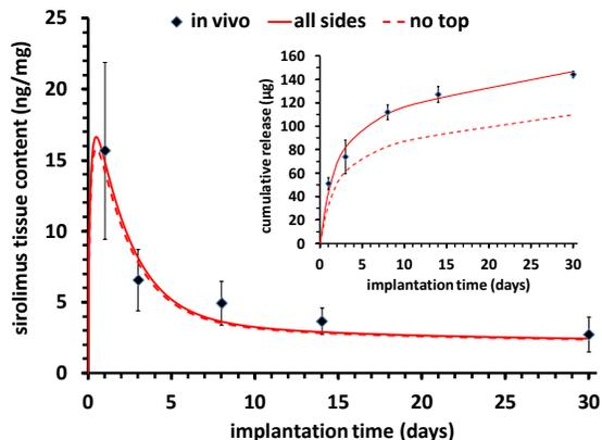
Figure 1. *In vivo* (diamonds) sirolimus tissue content and cumulative release (inset) versus model for fully coated struts (lines) and struts that are uncoated on lumen facing strut surfaces (dashes).
