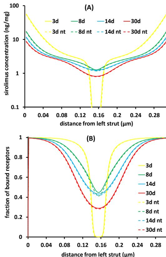
Figure 2. Predicted interstrut distribution of drug (A) and bound receptors for arteries stented with CYPHER (lines) or a hypothetical formulation that is uncoated on lumen facing strut surfaces (dashes, denoted as 'nt').
