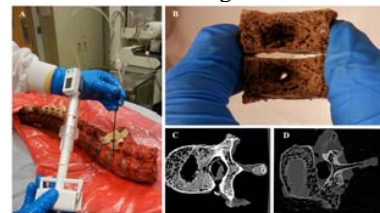
Figure 1. Creating simulated defects and filling with copolymers in cadaveric vertebral body. (A) Vertebral body defects were created using a lateral approach. (B) Picture of the simulated defect. (C) QCT scan showing the empty defect. (D) QCT scan showing the filled defect with P(PF-co-CL) copolymer.
