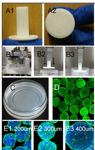
**Fig. 2:** High-speed robotic 3D islet-like structure fabricator developed in our lab that can generate uniform sized islet-like structures. Nuclei stained with DAPI for blue color and green for insulin antibody. Scale bar, 100 $\mu$ m.
