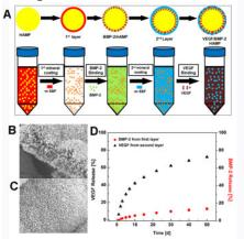
Figure 1. Schematic of dual release HAMPs fabrication (A) SEM image of the  $1^{st}$  layer (B) SEM image of the  $2^{nd}$  layer (C) Representative dual growth factor release profiles (D)
