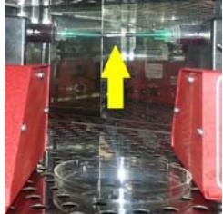
Figure 1. Blood perfusion setup for HFM. Arrow indicates HFM placed between collection chambers.
