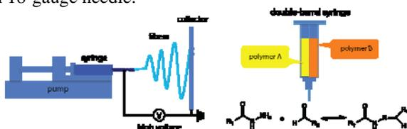
Figure 2. Scheme of electrospinning setup
