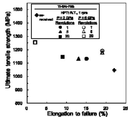
Figure 2. Ultimate tensile strength and Elongation to failure of Ti-6Al-7Nb before and after HPT processing
