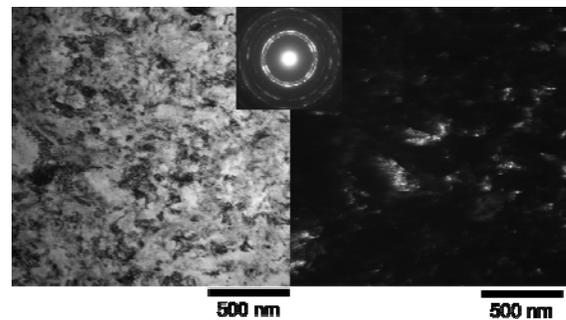
Figure 1. TEM image and SAED pattern of Ti-6Al-7Nb alloy processed by HPT under 6 GPa through 5 revolutions.
