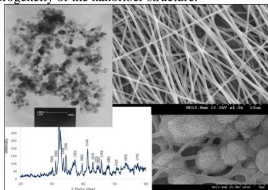
Figure1- TEM image and XRD pattern of bredigite nanoparticles and SEM images of PHBV nanofibers before and after immersion in SBF
