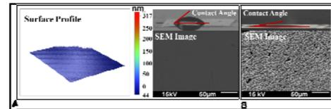
Fig.2. A) Surface characteristics of 0° chip including surface profile, SEM image and contact angle; B) SEM image and contact angle of 0° chip after 1hr chemical treatment
