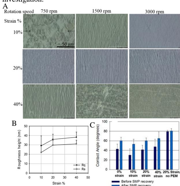
Figure 1. Material Characterization of PEM coated SMPs. A) Optical microscopy of PEM wrinkle patterns. The arrows indicate direction of compression. The scale bar is the same for all pictures. B) Substrate roughness analysis after SMP recovery. C) Contact angle analysis after SMP recovery.
