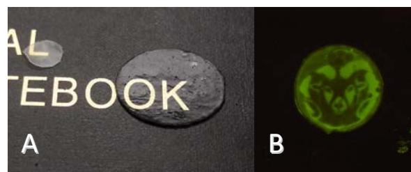
Figure 1. A Dry Polymer vs Swollen Hydrogel. B Photopatterned, fluorescently-tagged HA in hydrogel after 60 hour rinse in DI water.
