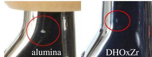
Figure 3: Representative femoral neck damage from static impingement and femoral head subluxation.
