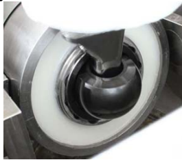
Figure 1: ASTM 2582:08 Neck impingement fixture
