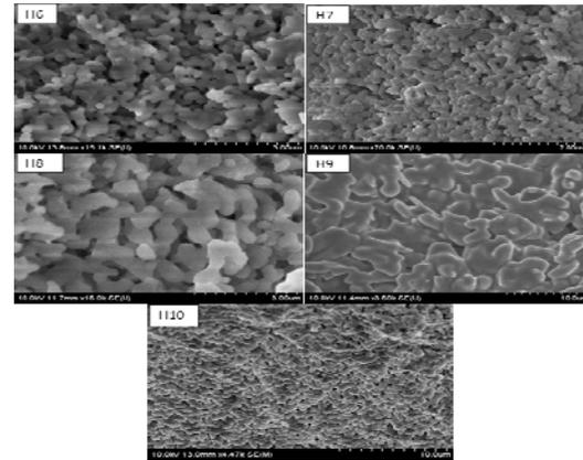
Fig 2 Microstructural evolution of  $\beta$ -T(Ca, Mg)P(H6, H7, H8), HA/ $\beta$ -T(Ca, P) (H10) with an average size of 2.7  $\mu\text{m}$  and MgP sintered (H9) with average particle size of 8.5 $\mu\text{m}$  when sintered at 1150°C.
