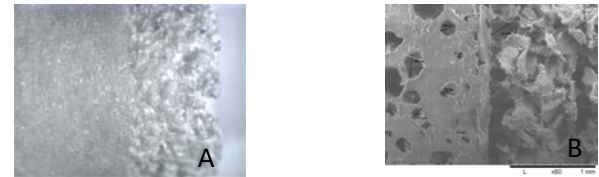
Figure 3. (A) Macroscopic image of the biphasic scaffold. (B) SEM image of the biphasic scaffold with visible pores ranging in size from 57 – 392 \mu m.
