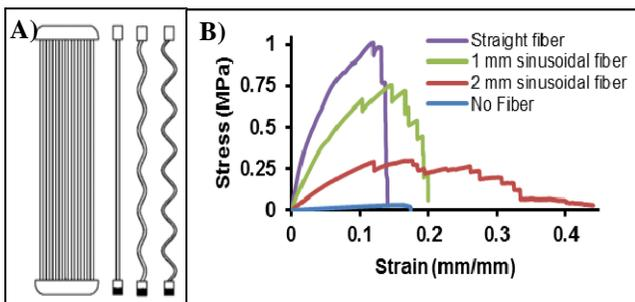
**Figure 1A)** Left to right: top view, side view of straight fiber, 1 mm amplitude sinusoidal fiber, and 2 mm amplitude sinusoidal fiber constructs. **1B)** Representative stress-strain curves of each fiber reinforced scaffold
