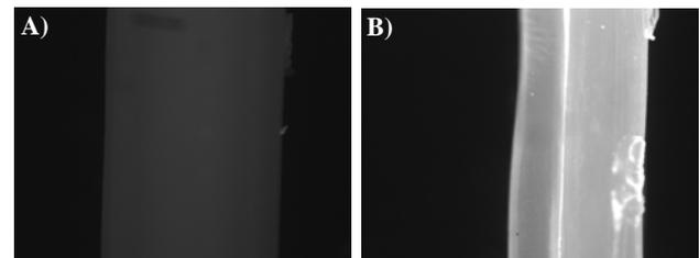
**Figure 2A)** ABS fiber without BSA functionalization (control) **2B)** ABS fiber functionalized with BSA via an oxygen plasma treatment
