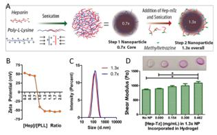
**Figure 1.** (A) Schematic of two-step sonication protocol for NP synthesis. Hep and/or Hep-mTz was added immediately before the second sonication step. (B) Zeta potential of NPs with varying [Hep]/[PLL] ratios at a constant [PLL] of 0.25 mg/mL. (C) Representative size distribution data. (D) Image and shear moduli of 3wt% PEG8NB-DTT hydrogels incorporated with modular NPs. NP-loaded hydrogels were swelled in DMMB for visualization of NP incorporation.
