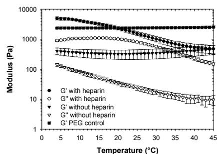
Figure 2. A plot of  $G'$  and  $G''$  as a function of temperature for dG-PBD gels with and without heparin and for PEGVS control gels ( $n=4$ ;  $\pm$ SD).
