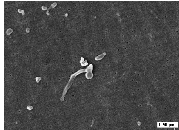
Figure 2: SEM micrograph of UHMWPE debris isolated from serum
