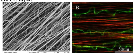
Figure 2: (A) SEM Image (B) Fluorescent Image of composite fiber matter with interlacing waved and straight fibers.
