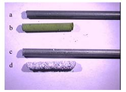
Figure 1. a. Fe rod; b. Fe in PBS for 1-week at 37 °C; c. Mg alloy rod; d. Mg alloy in PBS for 1-week at 37 °C.
