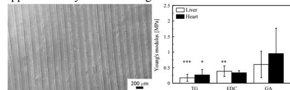
Figure 1. (Left) SEM image of liver dECM films with micropatterns. (Right) Young's modulus of dECM films. \*:  $p > 0.05$ , \*\*:  $p > 0.01$ , \*\*\*:  $p > 0.001$ , compared with GA.
