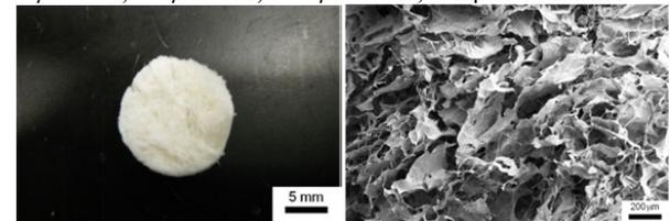
Figure 2. (Left) 3D porous liver dECM scaffold and (Right) its SEM image.
