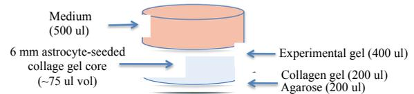
Figure 1. Migration assay setup consisting of a core astrocyte seeded collagen gel encapsulated within a collagen gel containing the experimental factors (genipin, LMTs, FGF-2 low: ~20ng/ml (low) high: ~200 ng/ml).
