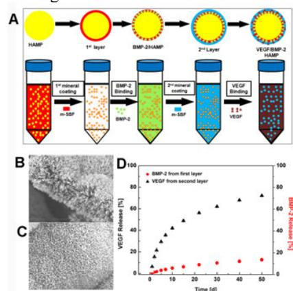
Figure 1. Schematic of dual release HAMPs fabrication (A) SEM image of the 1<sup>st</sup> layer (B) SEM image of the 2<sup>nd</sup> layer (C) Representative dual growth factor release profiles (D)
