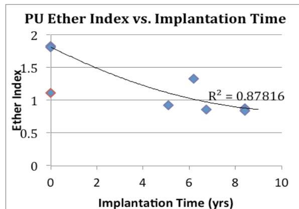
Figure 1. Ether Indices of Polyurethane leads based on ATR-FTIR spectra.
