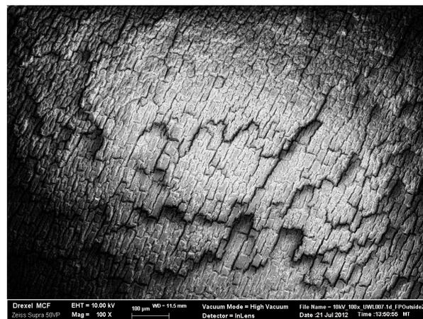
Figure 2. SEM image showing environmental stress cracking of a polyurethane lead.
