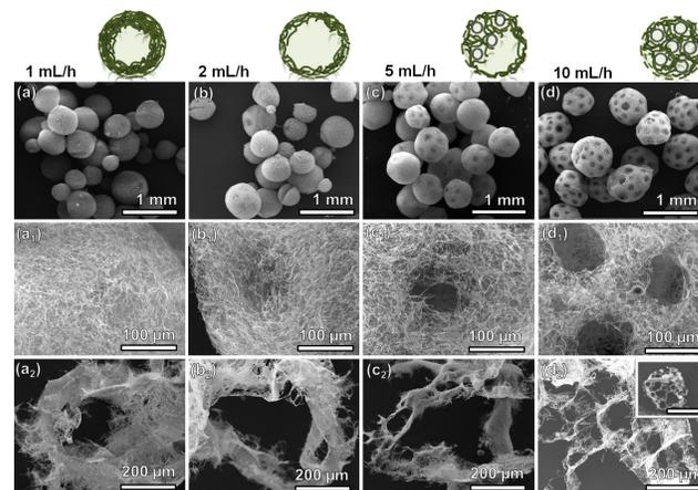
**Figure 1.** The effect of air flow rates on the formation of PCL:gelatin (1:1) NMs. (a-a<sub>2</sub>) 1 mL/h. (b-b<sub>2</sub>) 2 mL/h. (c-c<sub>2</sub>) 5 mL/h. (d-d<sub>2</sub>) 10 mL/h. The other processing parameters: short nanofiber concentration = 20 mg/mL, solution flow rate = 2 mL/h, applied voltage = 6 kV, distance between nozzle and collector = 10 cm.
