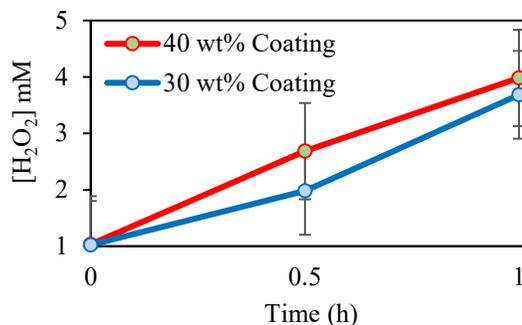
**Figure 1:** H<sub>2</sub>O<sub>2</sub> generation from polymer-coated PP fabrics upon hydration by pH 7.4 PBS.
