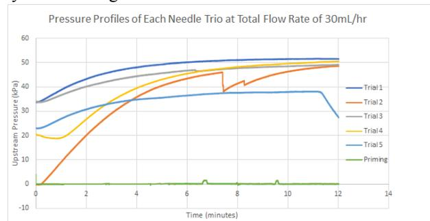
**Figure 2.** Pressure profiles for trials 1-5 and the priming process.
