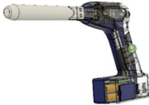
**Figure 1.** CAD rendering of the existing lead screw-driven ECE injector prototype.
