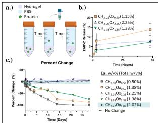
**Figure 2. Modified Hydrogel Optimization.** (a) Release schema. (b) BMP-2 release combinations. (c) Swelling over time with modified HA combinations.
