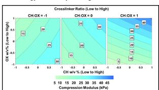
**Figure 1. Response Contour Compression Modulus.** Interaction between polymer concentration and crosslinker ratio.
