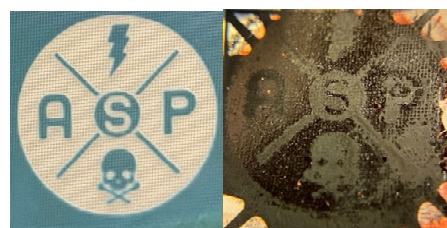
Figure 2. Screen mask and corresponding printed gelatin structure. Diameter of largest circle = 2.5 cm.
